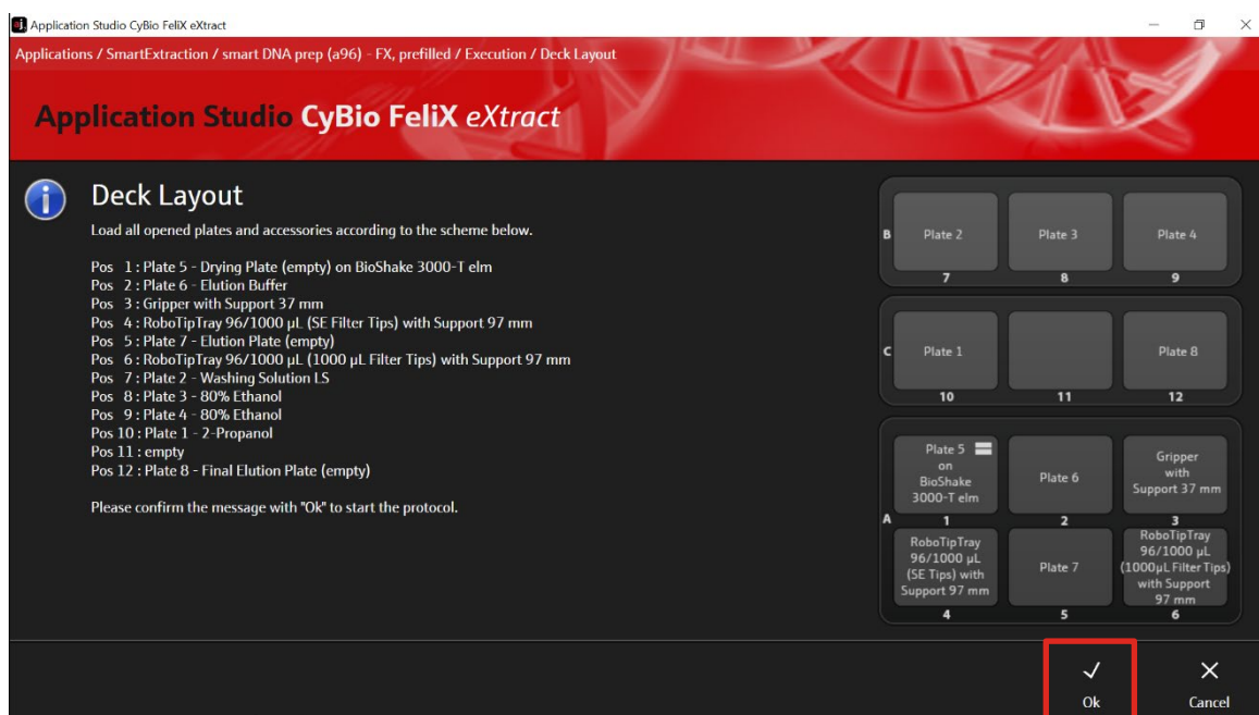
Figure 8: Deck layout for checking the correct positions of all plates and accessories.
