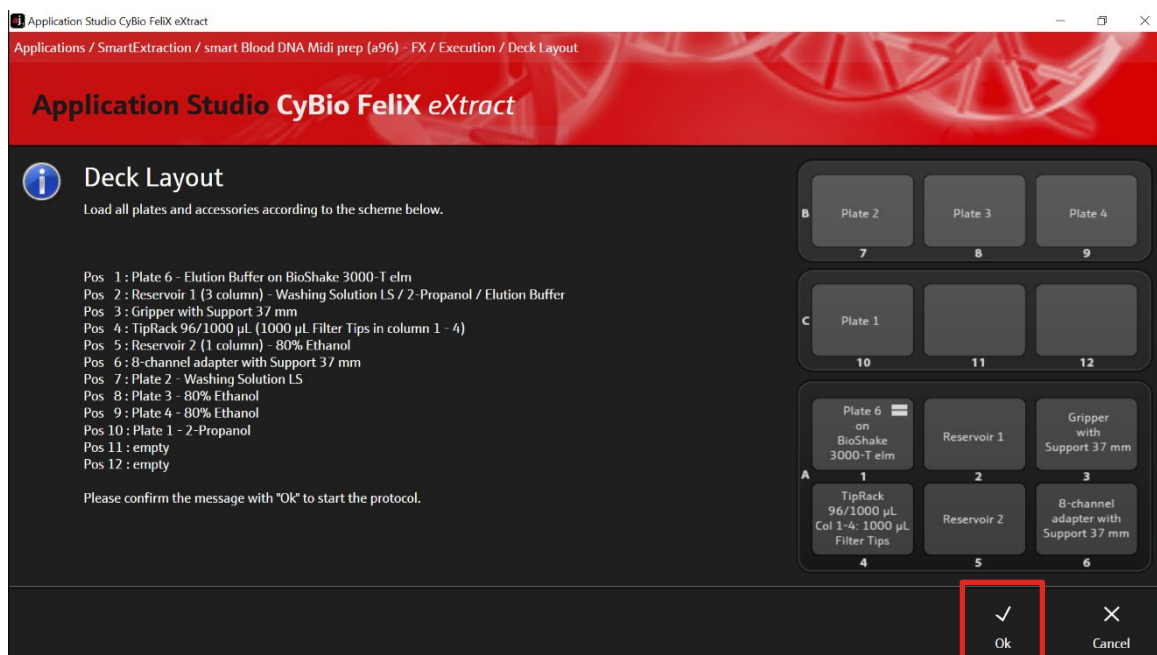
Figure 8: Deck layout for checking the right positions of all plates and accessories.
